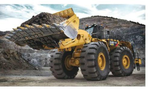
Cat's largest wheel loader—the 994H—applies 1,463 net hp (1,092 kW) of power and an operating weight of 431,000 lb (195,500 kg) to the task of loading large mining trucks up to the rated capacity of Cat's 240-ton 793D.
