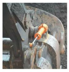
and gravity. Less damage to haul trucks is incurred because the door does not slam against the side of the bed when opening. Due to the smooth closing action, the dipper latch bar and dutchman insert also benefit by providing longer service life.
