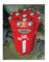
to **Rockmore International**. The CrossFlow design is intended to provide more efficient rock cutting flushing from the bit face, leading to better penetration rates and increased bit life. Because of the geometry and placement of flush holes, flush grooves and tungsten buttons, the bit can remove broken rock chips away from the bit face quickly, Rockmore International says.
