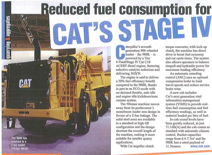
aterpillar's seventh generation 988 wheeled loader - the 988K - is powered by a Tier 4 Final/Stage IV Cat C18 ACERT diesel engine, featuring selective catalytic reduction and delivering 362kW.
