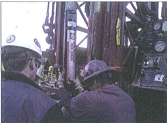
The ROK 500DH hammer mounted on a drill rig
