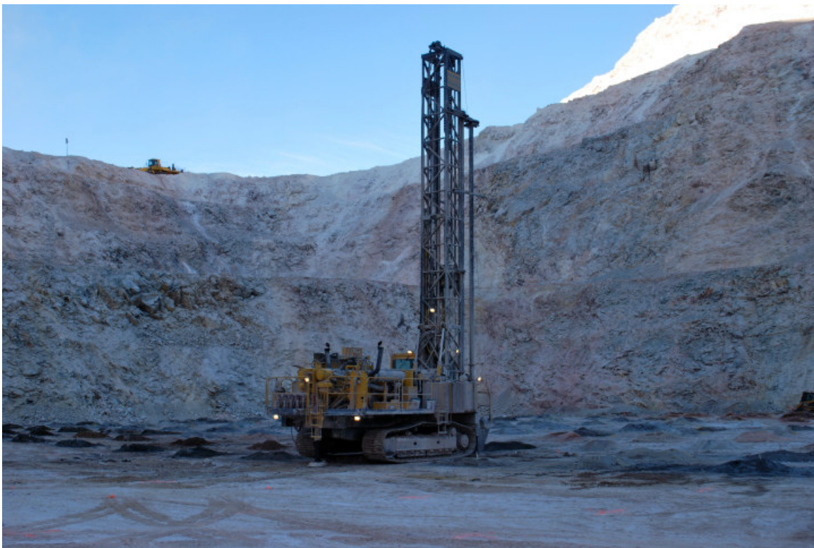
Drill Rig running a Rockmore ROK 650 Hammer and Rockmore DTH Bit in Nevada
