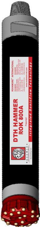
**SonicFlow Technology** greatly improves the air flow characteristics within the ROK hammer and ensures that the high pressure air paths are optimized to deliver greater energy to the piston. This is achieved by incorporating scientific air flow concepts in the design of the hammer and its various components such as the Top Sub, Piston, and Wear Sleeve. This technology results in more impact energy to the bit and produces higher penetration rates and better overall hammer performance.
