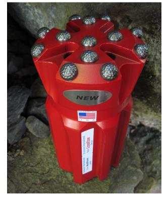
particularly in the geometry and placement of flush holes, flush grooves, and tungsten buttons. The intent of the new bit geometry is to remove the broken rock chips, that result from the percussive blows, away from the bit face and up towards the hole annulus as quickly and effectively as possible.
